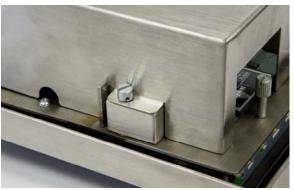
Figure A-18: Internal Sealing, Revised PCB
