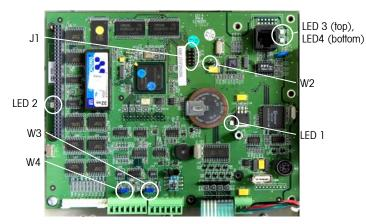
Figure A-13: Jumper and LED Locations, Original Main PCB
