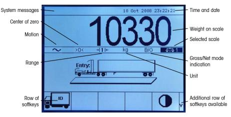
Figure 2-6: Default Vehicle ID Weighing Operation Screen
