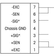
\*If an increase in load results in a decrease in weight display, reverse the signal wires (+SIG and -SIG).
