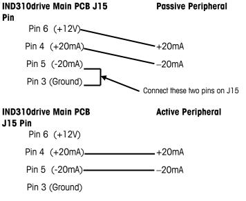
Figure A-12: Connecting the Current Loop to Passive and Active Peripherals
