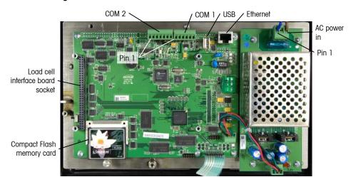
Figure A-4: PCB with Associated Connectors
