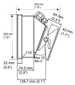
Figure 1-3: Side View of IND310drive
