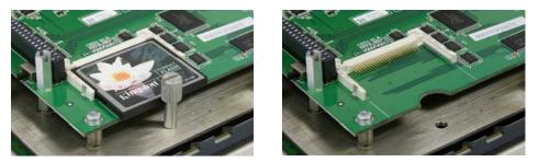
Figure 4-4: Compact Flash Card (METTLER TOLEDO Part No. 72225800)
