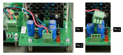
Figure 4-5: Pins 1, 2, and 3 on the Power Supply Board
