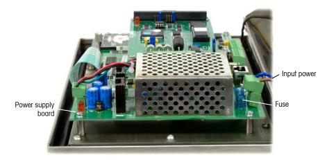
Figure A-5: Power Supply Board
