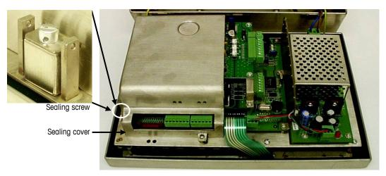
Figure A-17: Internal Sealing, Original PCB
