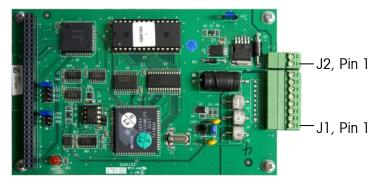
Figure A-9: POWERCELL Board Connector Locations
