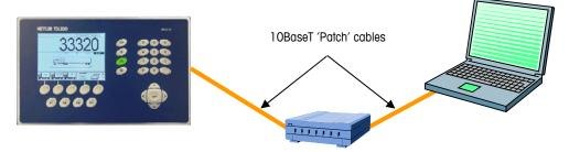
Figure B-2: Connecting the IND310drive to a PC with Patch Cables
