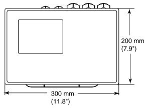
Figure 1-2: Top View of IND310drive
